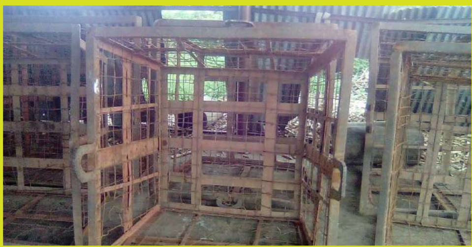
Hot water treatment trays
